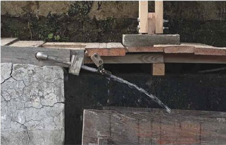
Wood and metal water spout system, to provide adjustable pressure of water
